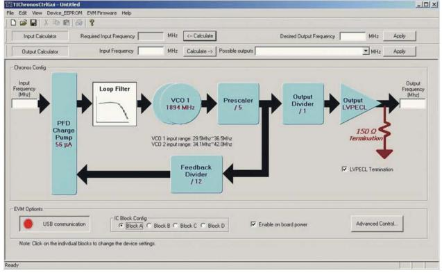
Figure 5. TI Chronos Software GUI
